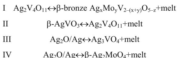
Points  $\Delta\text{T}'\text{-}2$ ,  $\Delta\text{T}'\text{-}3$  and  $\Delta\text{T}'\text{-}6$  are pseudo-triple points. They correspond to the final stage of meritecic reactions I–IV.
