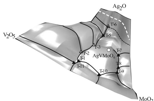
**Fig. 2** Three dimensional presentation of  $\text{V}_2\text{O}_5-\text{MoO}_3-\text{Ag}_2\text{O}$  diagram drawn by the AutoCAD programme. The full lines show boundary curves, the triangles show ternary and ‘pseudo-ternary’ eutectics
